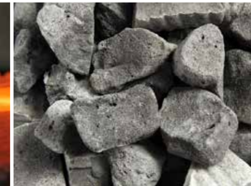
Upon cooling, the foam glass cake breaks through tension cracks into foam glass gravel.
