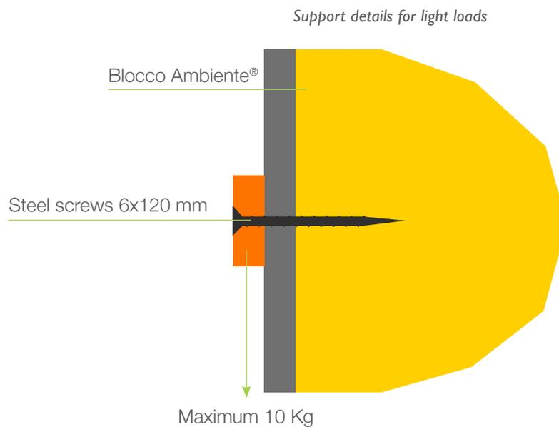
In case of heavy loads, insert mechanical anchors or threaded bars downed in epoxy resin or rapid cement, for minimum 10cm depth.
