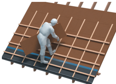
Application without breathable membrane.
